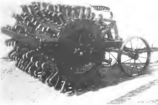
A Tamping Roller Showing the Feet of the Iron Sheep.
